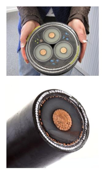
The submarine cable and onshore cable used in the Vineyard Wind project. Two pairs of submarine cables will connect 1600 megawatts of renewable offshore wind energy to land. The cables will be buried within a 35 mile corridor from the turbines to shore. Multiple cables are necessary to transmit the power and ensure reliability.
